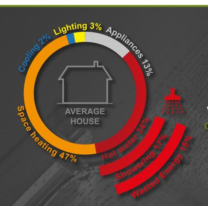
"Around 15% of energy used in the average UK home goes **down the drain** as waste shower water. Recoup WWHRS captures that energy and reuses it.
