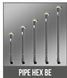
WWHRS is a simple fit-and-forget technology with no electrical components, no pumps or controllers, and so it requires very little maintenance. It also does not impact end-user shower experience and is normally hidden from view. Vertical WWHRS systems such as the Recoup Pipe+ HE are required to install on the floor below the shower(s) they attach to, and as such as an ideal solution for new build houses or commercial projects with service risers.
