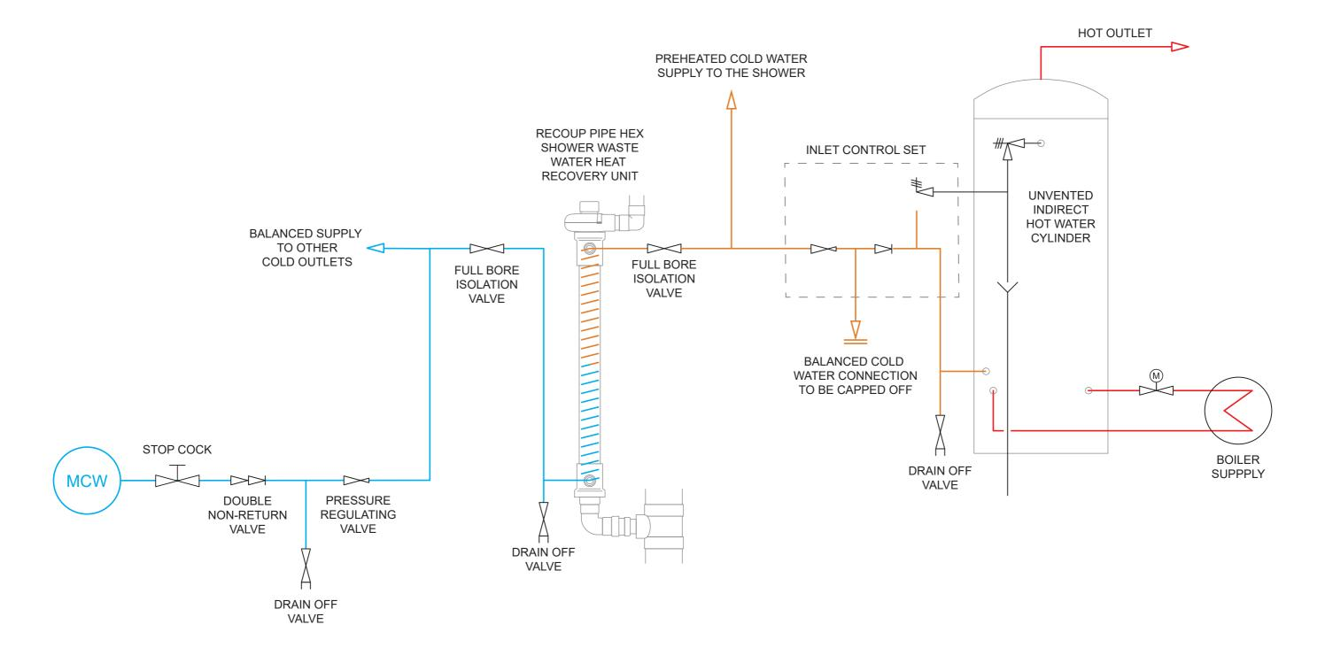
These drawings are specific to Waste Water Heat Recovery for Showers (WWHRS). Recoup Energy Solutions Ltd do not hold any responsibility for the design or M&E integration of WWHRS to the cold water services. It is the responsibility of the installer to read the specification and installation instructions.
