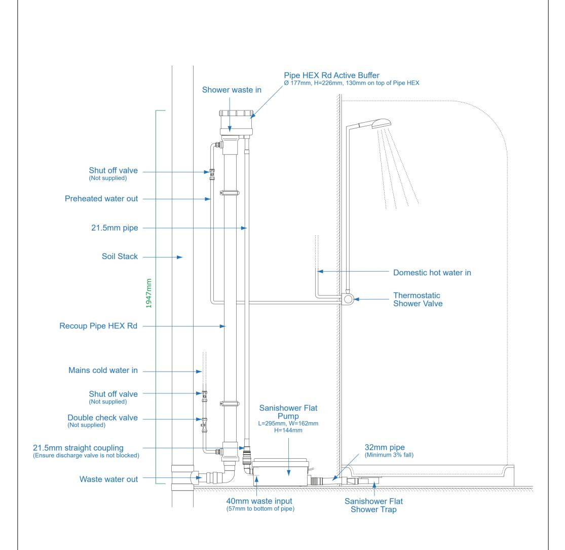
These drawings are specific to Waste Water Heat Recovery for Showers (WWHRS). Recoup Energy Solutions Ltd do not hold any responsibility for the design or M&E integration of WWHRS to the cold water services. It is the responsibility of the installer to read the specification and installation instructions. WWHRS drawings and installation documentation must be adhered to. THIS DRAWING REMAINS THE PROPERTY OF RECOUP ENERGY SOLUTIONS LTD.
