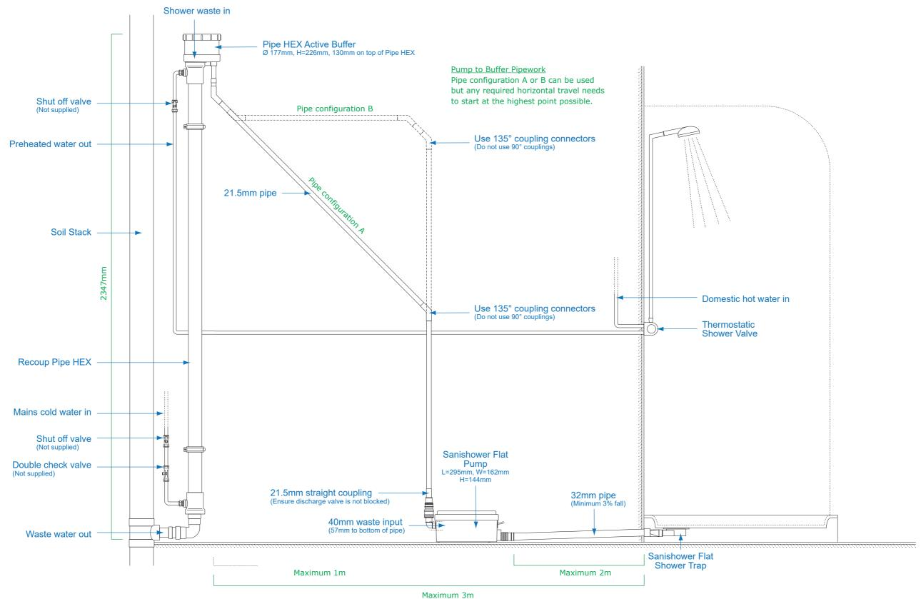
These drawings are specific to Waste Water Heat Recovery for Showers (WWHRS). Recoup Energy Solutions Ltd do not hold any responsibility for the design or M&E integration of WWHRS to the cold water services. It is the responsibility of the installer to read the specification and installation instructions. WWHRS drawings and installation documentation must be adhered to. THIS DRAWING REMAINS THE PROPERTY OF RECOUP ENERGY SOLUTIONS LTD.
