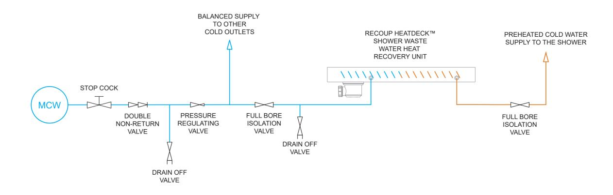
These drawings are specific to Waste Water Heat Recovery for Showers (WWHRS). Recoup Energy Solutions Ltd do not hold any responsibility for the design or M&E integration of WWHRS to the cold water services. It is the responsibility of the installer to read the specification and installation instructions.
