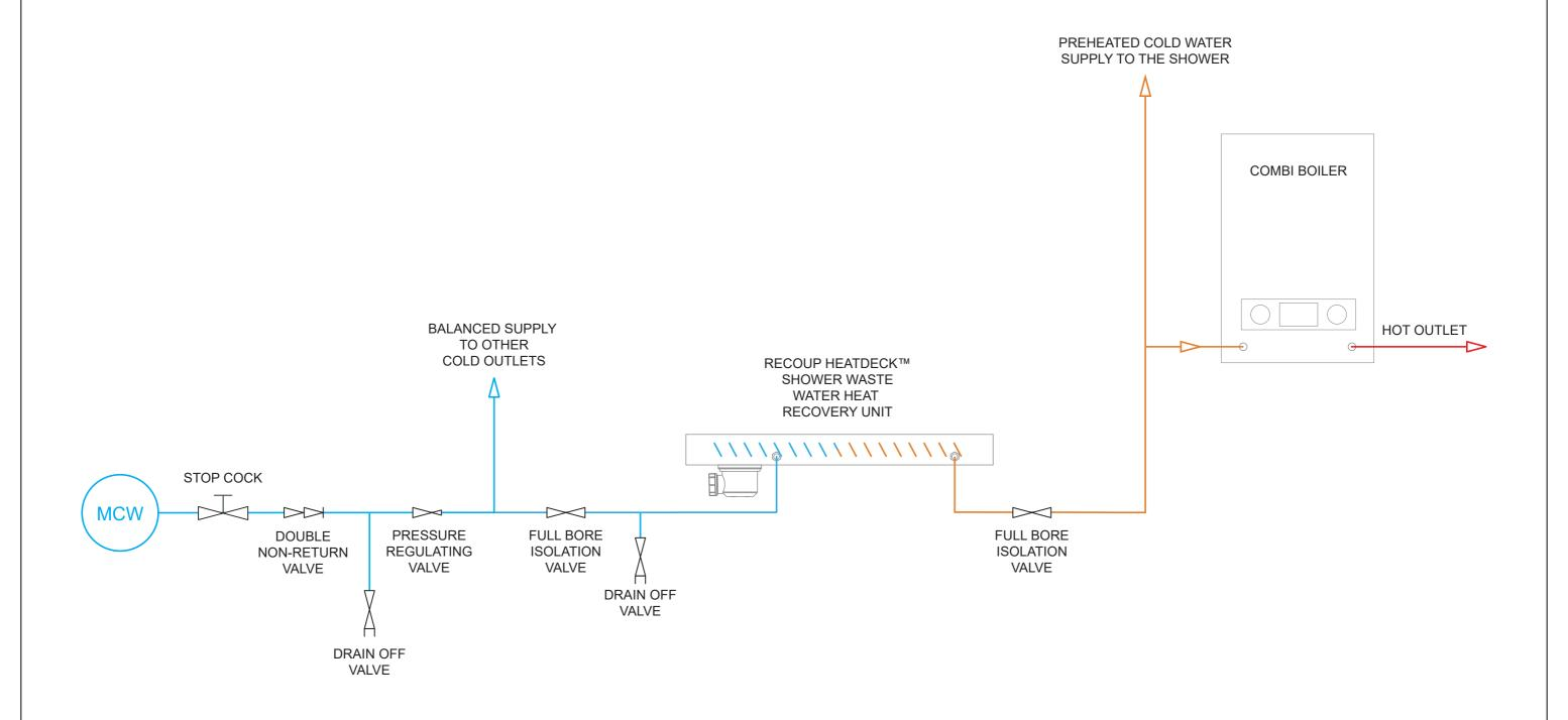
These drawings are specific to Waste Water Heat Recovery for Showers (WWHRS). Recoup Energy Solutions Ltd do not hold any responsibility for the design or M&E integration of WWHRS to the cold water services. It is the responsibility of the installer to read the specification and installation instructions.
