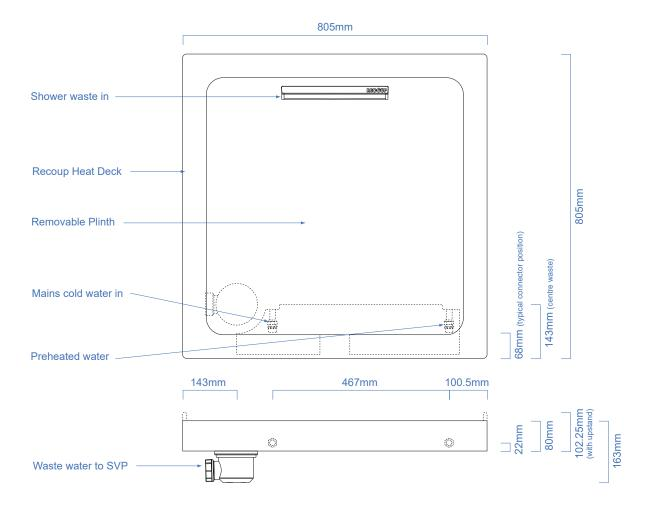
These drawings are specific to Waste Water Heat Recovery for Showers (WWHRS). Recoup Energy Solutions Ltd do not hold any responsibility for the design or M&E integration of WWHRS to the cold water services. It is the responsibility of the installer to read the specification and installation instructions.
