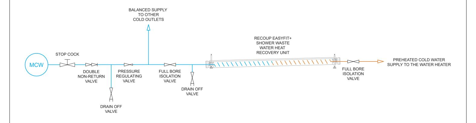
These drawings are specific to Waste Water Heat Recovery for Showers (WWHRS). Recoup Energy Solutions Ltd do not hold any responsibility for the design or M&E integration of WWHRS to the cold water services. It is the responsibility of the installer to read the specification and installation instructions.
