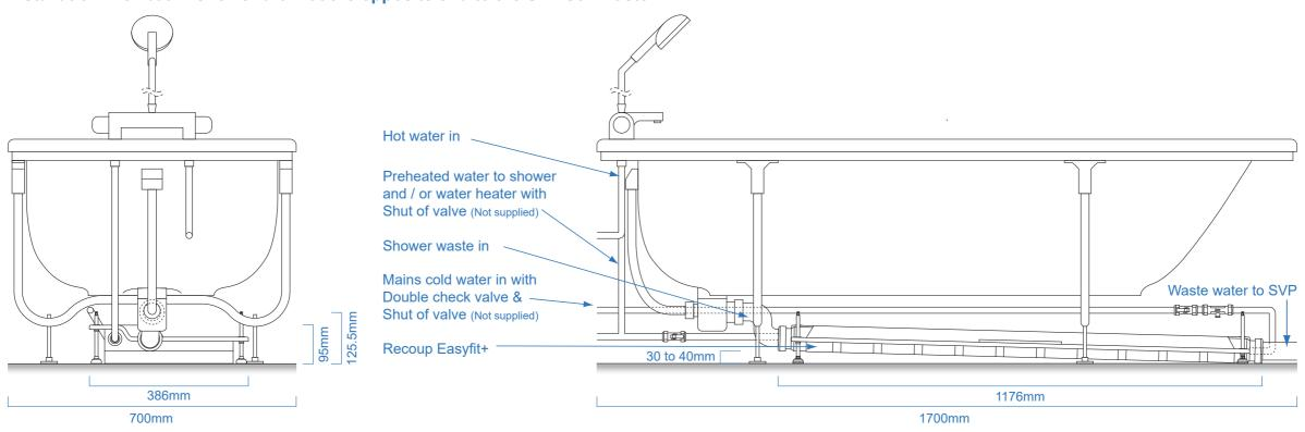
These drawings are specific to Waste Water Heat Recovery for Showers (WWHRS). Recoup Energy Solutions Ltd do not hold any responsibility for the design or M&E integration of WWHRS to the cold water services. It is the responsibility of the installer to read the specification and installation instructions.
