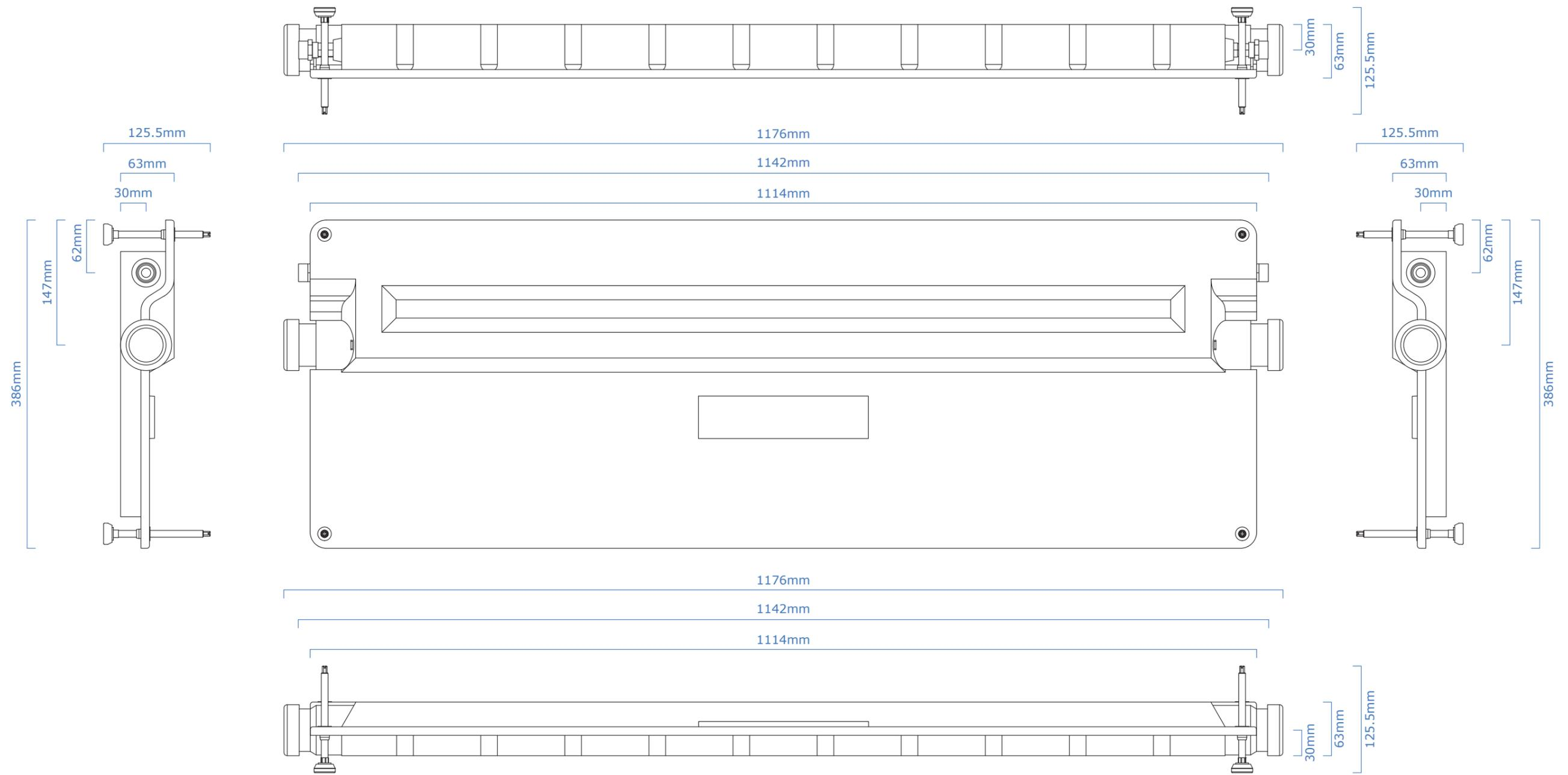
These drawings are specific to Waste Water Heat Recovery for Showers (WWHRS). Recoup Energy Solutions Ltd do not hold any responsibility for the design or M&E integration of WWHRS to the cold water services. It is the responsibility of the installer to read the specification and installation instructions. WWHRS drawings and installation documentation must be adhered to. THIS DRAWING REMAINS THE PROPERTY OF RECOUP ENERGY SOLUTIONS LTD.
